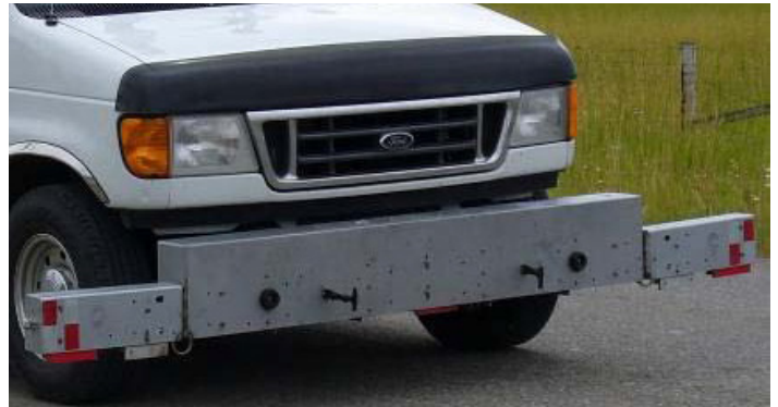
Data from high-speed pavement survey equipment is fed into on-board computers when portions of the road network are surveyed – Ministry of Transportation and Infrastructure photo
