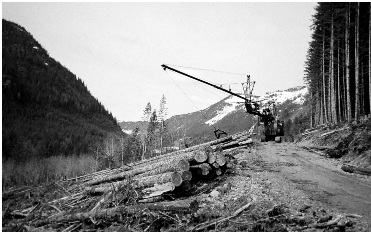
A lone operator casts a grapple downslope to retrieve felled timber. (OAG staff photo)
